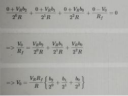
Substituting,  $R=2R_f$  f in above equation.
