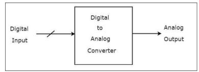
A Digital to Analog Converter (DAC) consists of a number of binary inputs and a single output. In general, the number of binary inputs of a DAC will be a power of two.
